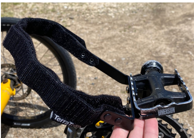
Standard pedal with adjustable heel strap, found mostly with our recumbent trikes
