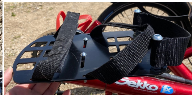
Adaptive foot pedals with ankle and toe straps, found on our recumbent trikes
